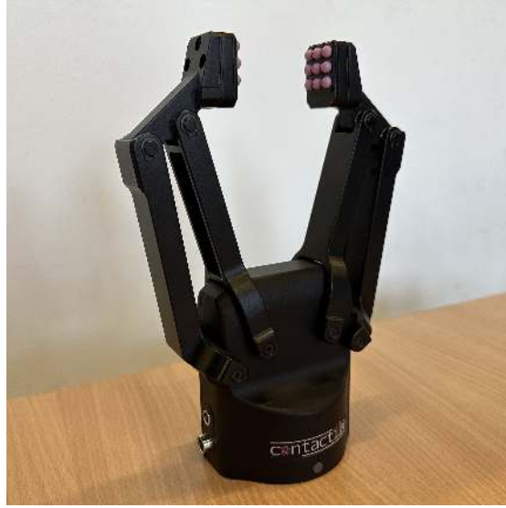
Fig. 1. Robotic manipulator (Contactile GAL2 Gripper) equipped with the Contactile PapillArray sensors.
