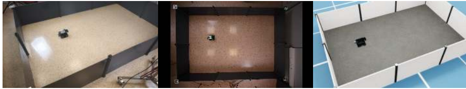
Fig. 2: Robot position viewed from outside the arena (left), from the overhead camera (middle), and in its final position in Isaac Sim (Right).
