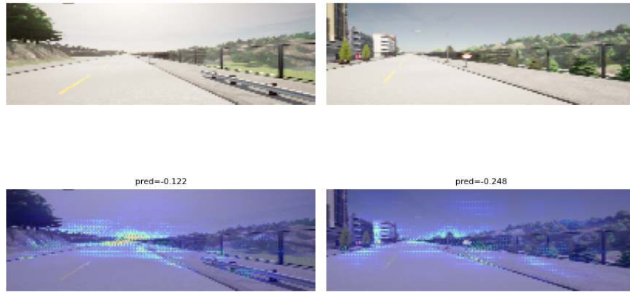
Fig. 4. Two input images, not cropped, and the focus of attention of the model on them according to SHAP.
