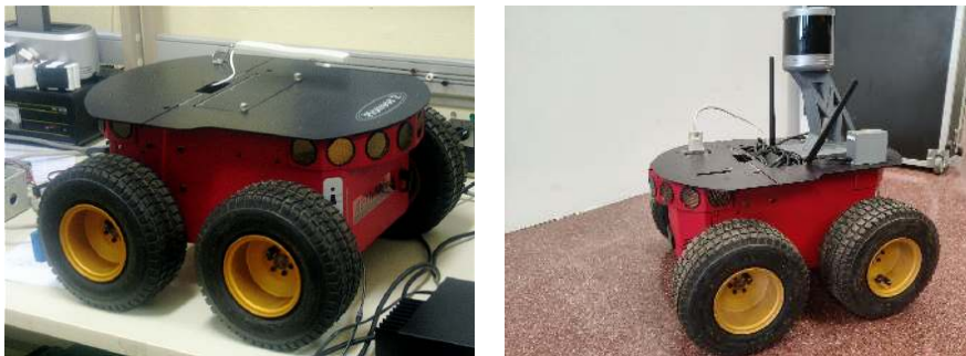
Fig. 1. Before/after of the retrofit. Left: the original Pioneer 2-AT. Right: the retrofitted robot.
