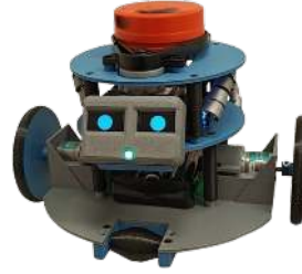
Fig. 2. The re-engineered Robotito (final PCB revision), with managed wiring, modular PCB and the audiovisual HRI module.
