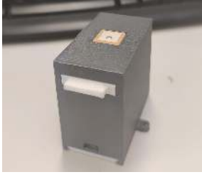
Fig. 4. The printed enclosure housing of the Air530Z GNSS.
