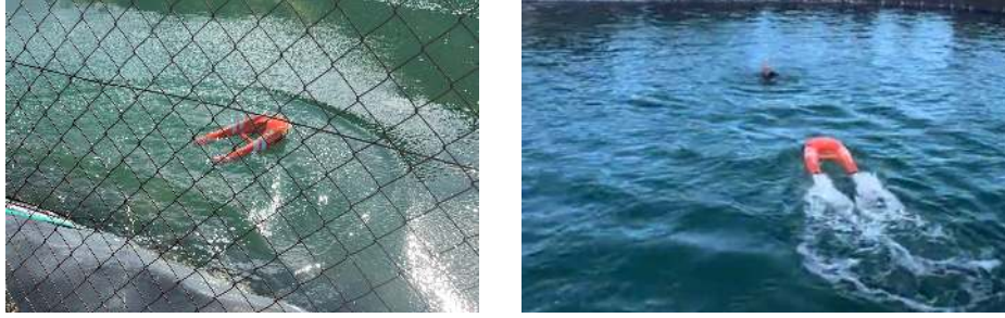
Fig. 1: (Left) The self-propelled rescue buoy ( hover ) under test on the target reservoir, seen through the perimeter fence; the geomembrane lining is visible at the bottom left. (Right) The robot is approaching to the person. Normally driven by a 433 MHz hand-held remote, here it is commanded by a cloned radio link.
