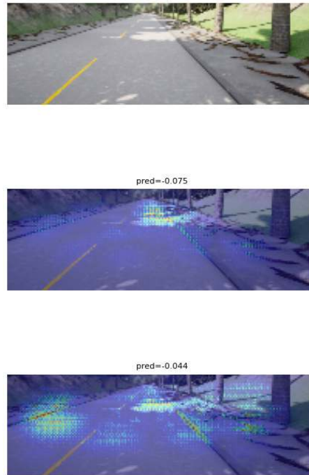
Fig. 5. Initial images (top); focus of attention in regular dataset (middle row); and training with Two-weather-conditions dataset (bottom row).
